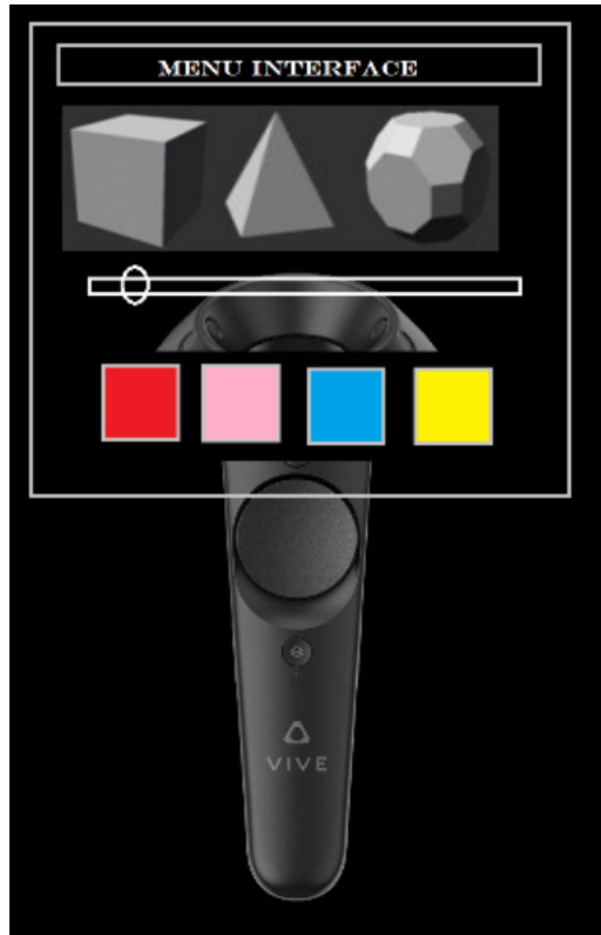
Figure 2. The UI menu that features the primitive and color options as well as the size slider. This menu will hover over the controller as a diegetic UI component
